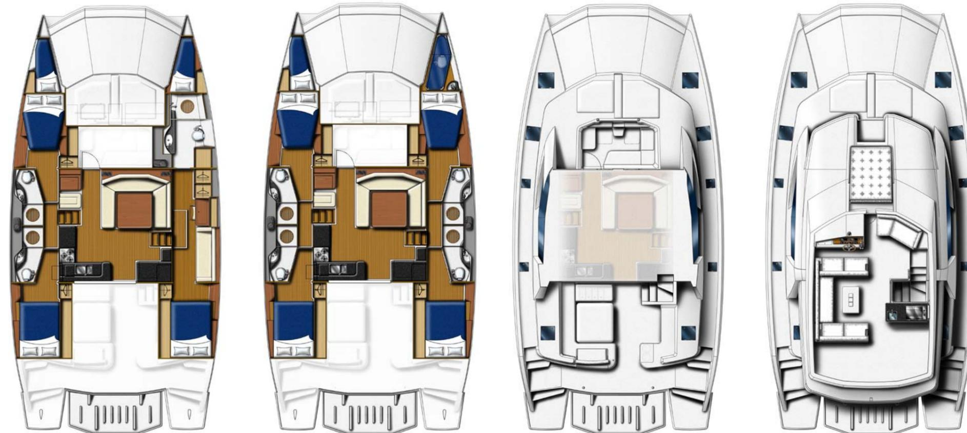
The Leopard 51 Powercat is available in either a 3 cabin, 3 head version, or a 4 cabin, 4 head version. Both layouts offer the option of additional storage, berth, or head in the forward hull.
