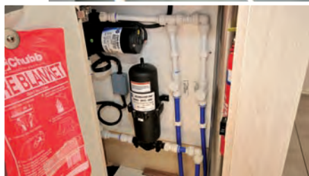
Easily understood plumbing, with fresh water pressure pumps grouped together in a galley locker. I liked the thermo-engraved labeling
