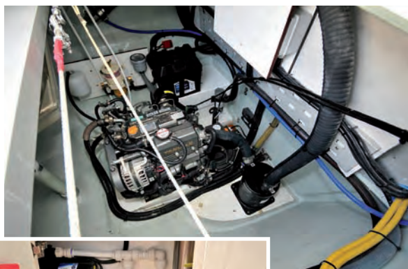
Maintenance access is ok for someone not too big. Note the filters and coolant reservoir mounted on a laminate panel rather than being screwed into the composite
